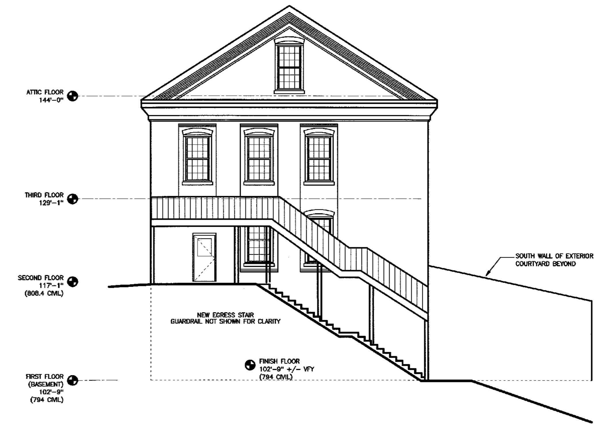
21 CHAMBERLIN (SOUTH BUILDING) SOUTH ELEVATION 1/8" = 1'-0"
