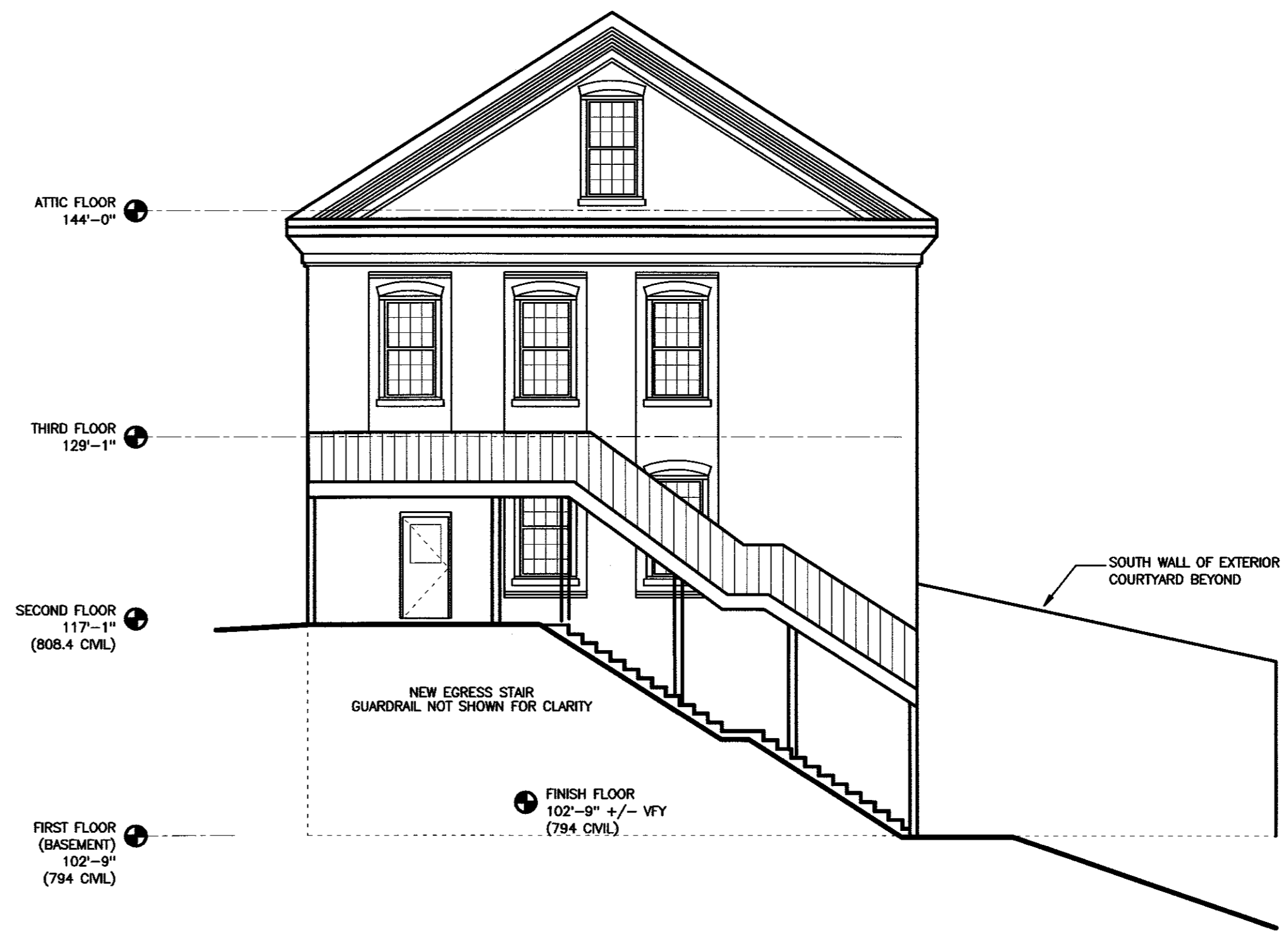
21 CHAMBERLIN (SOUTH BUILDING) SOUTH ELEVATION 1/8" = 1'-0"
